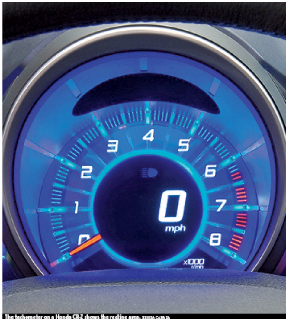
The tachometer on a Honda CR-Z shows the redline area. EDINA CARL DA
